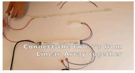
For video instructions on how to setup BIOS Linear Arrays with BIOS Production Bio-Dimming Modules scan this QR Code.
