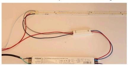
Step 5. Turn ON lights at MAXIMUM POWER. Leave maximum power for at least 10 seconds. Lights will flash to the warm channel and then back to the cool channel.
